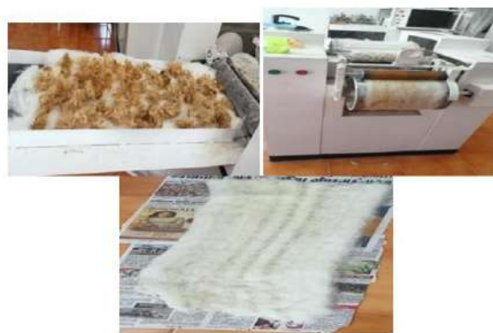
Figure. 12: (a): Arranging the extracted fibers in carding machine (b): Lap formation of natural fibers with ratio 70:30 (areca and Cotton) (c): Formed composite fiber lap
